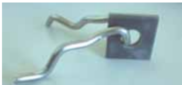
Rotary Kiln Anchors A 'V' tack welded to a square cleat, which is welded to the casing.
