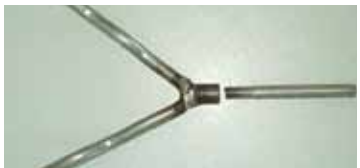
Y-Anchors 2 part anchor for multi-component linings. The stud part of the anchor will retain back-up layers of board, whilst the V can anchor castable.
